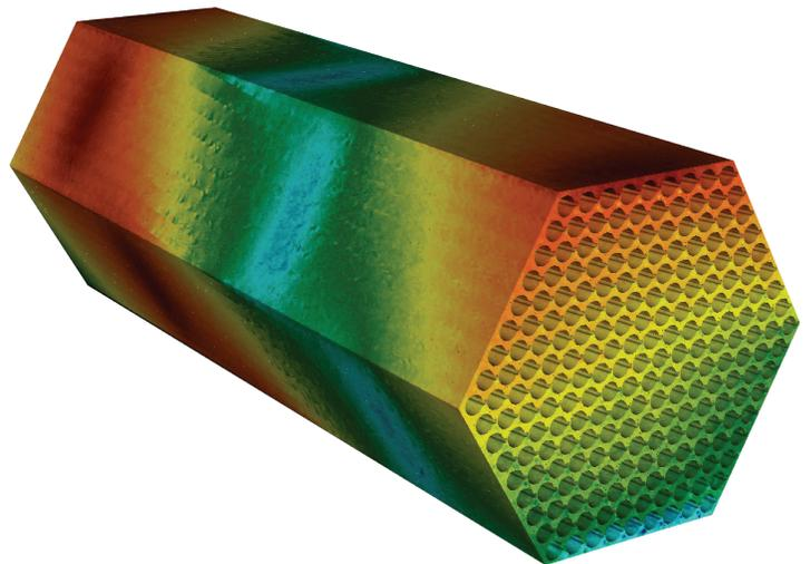
*Pressure distribution for turbulent coolant flow in a 217-pin nuclear reactor subassembly. The simulation was performed by the Argonne SHARP (Simulation-based High-efficiency Advanced Reactor Prototyping) group using 32,000 processors of the Blue Gene/P at the Argonne Leadership Computing Facility. Computer time was provided through the DOE INCITE program.*
