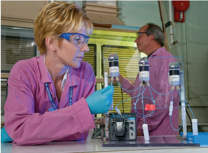
*Physical Chemist Carol Mertz (left) and Analytical Chemist Mike Kalensky use the mini-Gas Pressurized Extraction Chromatography (GPEC) system to age date radioactive source materials. Argonne has developed and validated age-dating methods and guidance documents for the entire nuclear forensics community using the GPEC system and other separation and analysis technologies.*
