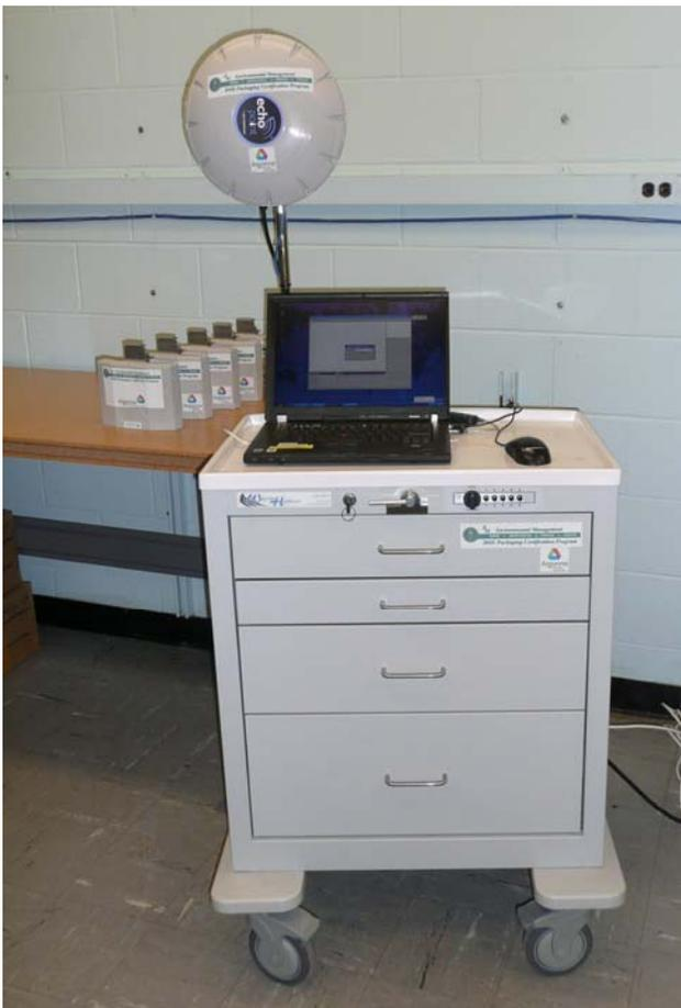
**FIGURE 4. A complete RFID monitoring system on a compact, mobile platform**
