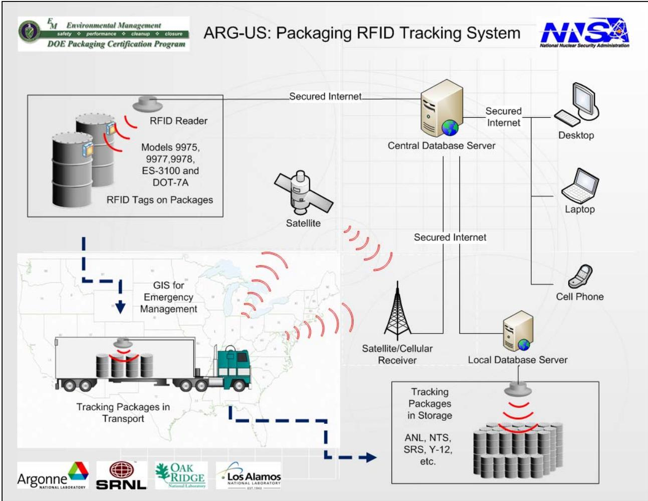
FIGURE 1. Concept of packaging RFID monitoring and tracking system for nuclear materials management
