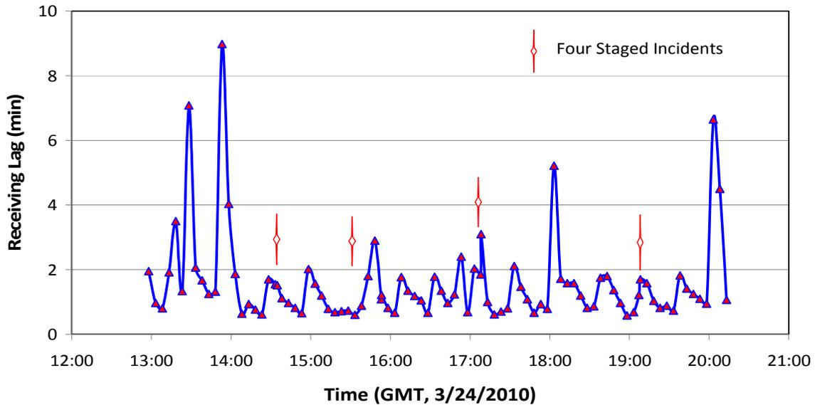
**Figure 5.** Time lag in receiving messages during the road test of the truck
