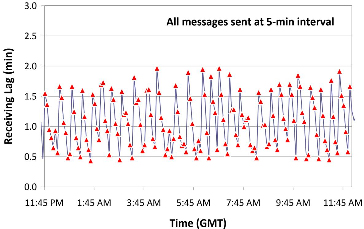
**Figure 3.** Typical time lags between send and receipt in stationary tests
