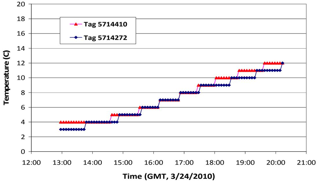
**Figure 6.** Temperature data from two of the tags in the truck during the road test. The gradual increase in temperature occurred because the test started at  $\approx 8$  am local time.
