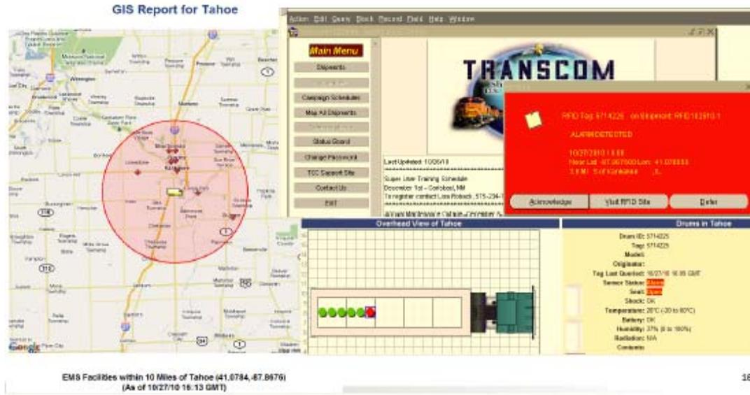
**Figure 8.** Screens appearing after alarm detected in the TRANSCOM/ARG-US RFID system
