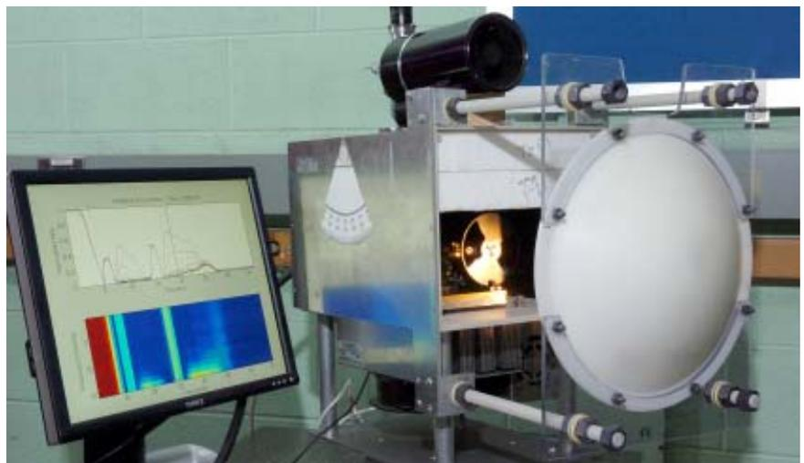
*A prototype of the passive millimeter-wave spectroscope.*
