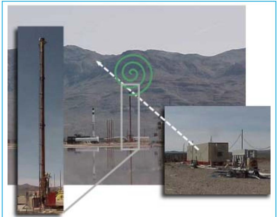
*Tests of the millimeter-wave spectroscope were conducted at the Nevada Test Site, shown here. Housed in a bunker (inset, right) several hundred meters from the test site (center), the spectrometer was able to distinguish the signal of gas plumes (represented by the green spiral) from the background mountains.*
