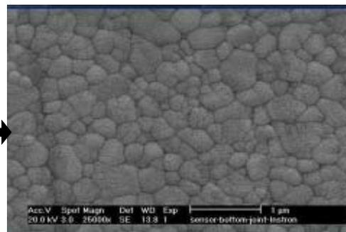
*The area between the arrows is the interface of two YSZ (yttria stabilized zirconia) components which comprise an oxygen sensor. The Argonne Plastic Joining Process results in a monolithic structure - note the interpenetrating grains with no porosity at the interface (shown by the arrows)*
