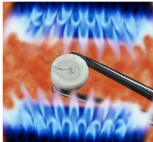
*Oxygen sensor designed by Ohio State University and fabricated using Argonne National Laboratory's unique plastic deformation process.*
