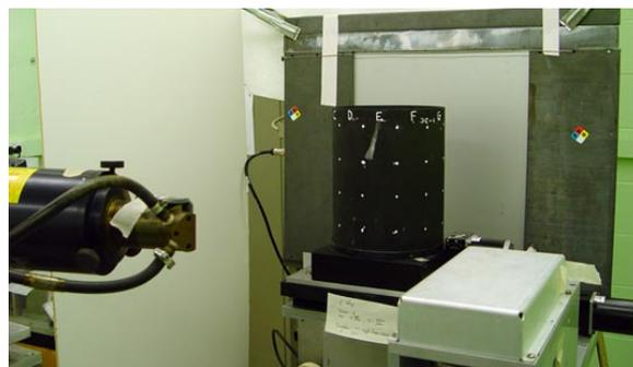
**OMX-161 source (left) with PerkinElmer RID detector (behind lead shield). A carbon composite sample is located on the 3-axis controlled stage in front of the detector.**
