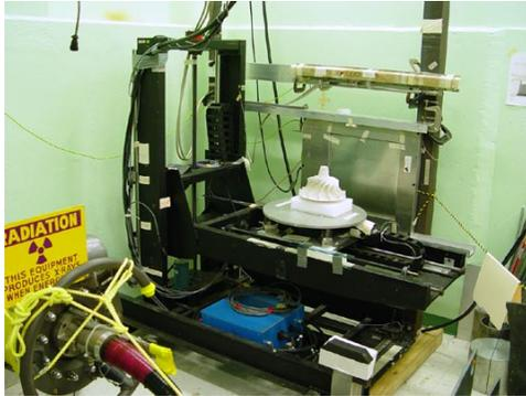
*Philips MG-450 source with RID area detector and CMOS linear detector (above RID). A prototype ceramic rotor is shown on the Multi-Axis controlled stage (in front of RID detector)*
