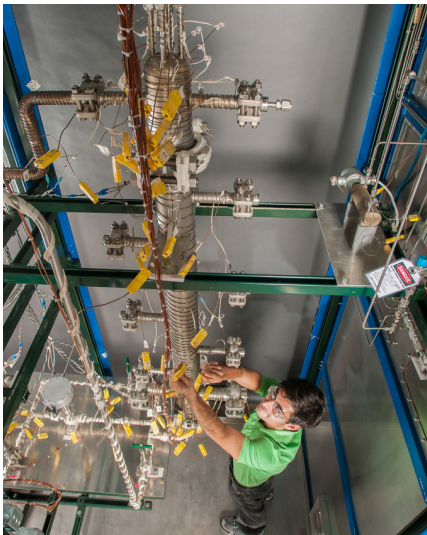
Argonne's SNAKE facility is used to study the effects of S-CO 2 leakage within advanced reactor heat exchangers.
