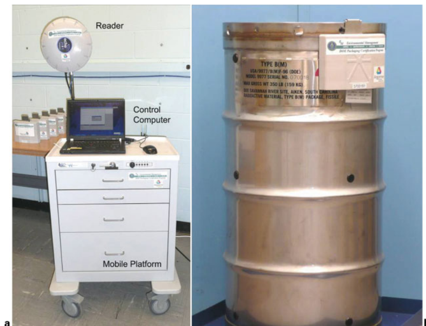
2 a stand alone RFID temperature monitoring system on mobile platform and b RFID tag mounted on 9977 (or 9978) package
