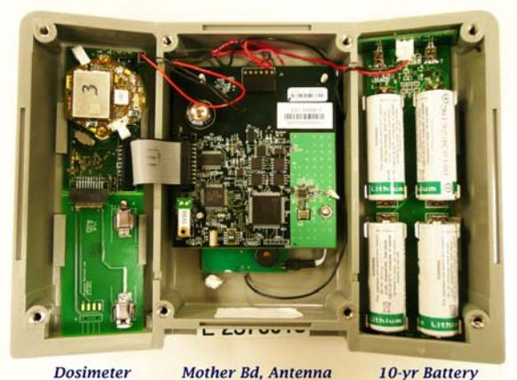
**FIGURE 3. Construction of ARG-US RFID tag**
