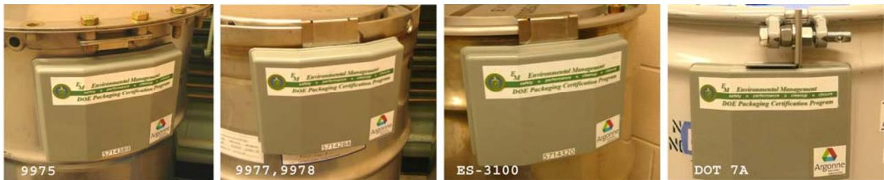
FIGURE 2. ARG-US RFID tags mounted on multiple drum types
